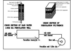
**DETAILS OF RAIN WATER HARVESTING STRUCTURES**
